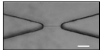
A microfluidic device is custom-designed in our group in order to form stable freestanding membranes. A picture of the membrane is shown.
